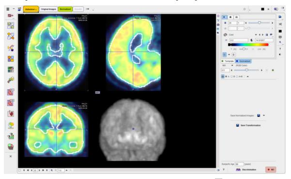
Initially, the color tables are applied which were defined in the <u>configuration</u> panel. To change the color tables or the thresholds please activate either the **Template** or the **Normalized** tab, and adjust the settings according to your preference.
