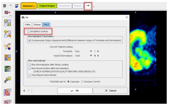
Simplified controls allows switching between the two processing modes. In the COLOR TABLES section the default color tables of the stereotactic Template and the subject images (Input & Normalized) can be defined. If the View Report automatically box is checked, the report viewer will be started each time a discrimination analysis is completed.
